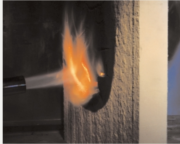
Propane test on PIR insulation core, after 3 hours
